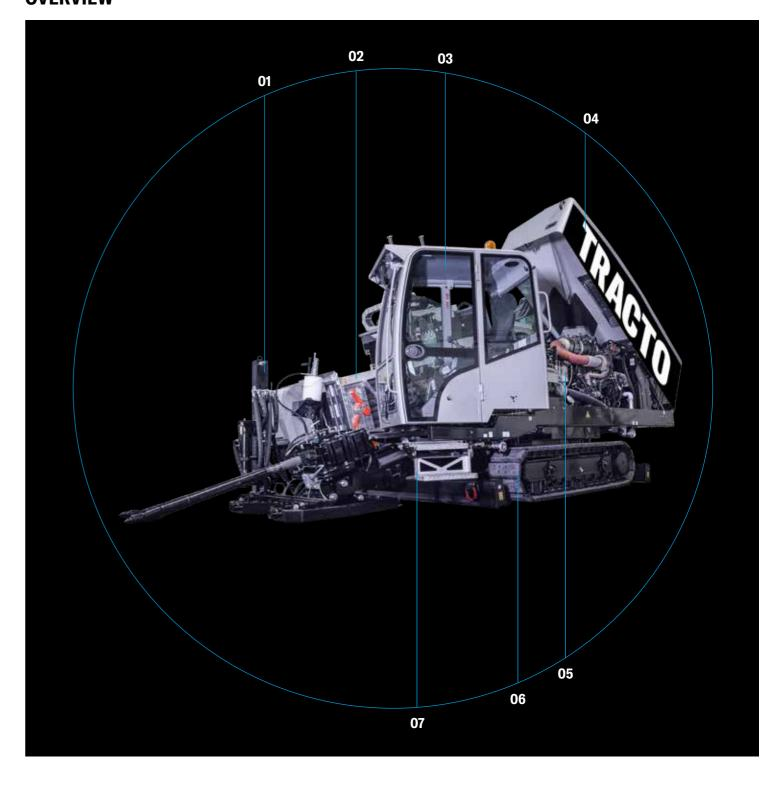
**O1 Anchoring system** for increased stability while drilling
